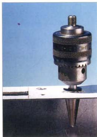
Fig. 5: A 'spare' 10mm chuck from a power drill make a good handle for a fluted reamer up to 20mm diameter.
