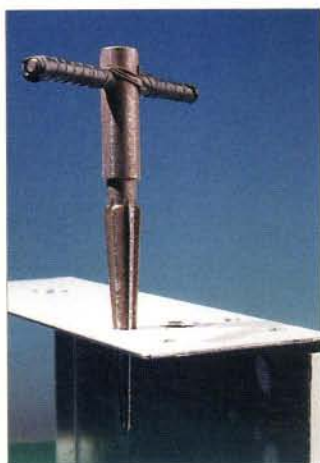
Fig. 4: A fluted reamer is useful for circular holes up to 12mm diameter.
