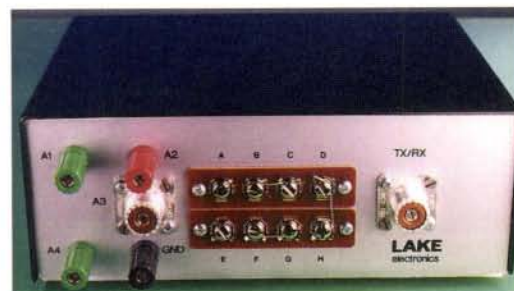
Fig. 9: Several configurations are possible using the 'patch panel' on the rear of the TU4 unit. Both balanced and unbalanced output are possible with the unit.
