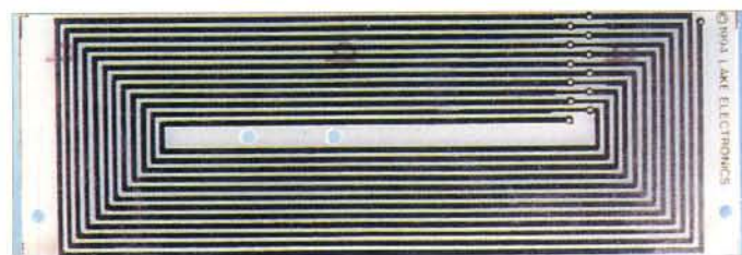
Fig. 6: The p.c.b. coil used in the Lake Electronics TU4 antenna tuner.
