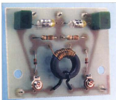
Fig. 7: The s.w.r. sensing board included in the TU4 a.t.u.
